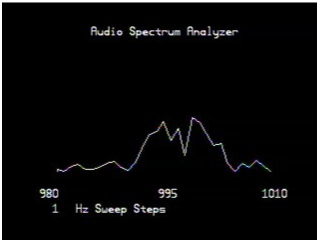
This image illustrates the bandwidth limitation. Here, the data was sampled for 100 Periods with an input frequency of 995Hz and 1000Hz. The sweep step was set at 1Hz intervals between 980Hz and 1010Hz
