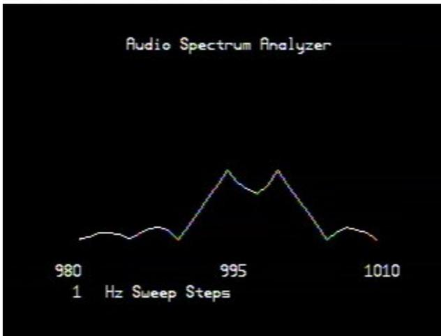
In this image, the data was sampled for 1000 Periods with an input frequency of 995Hz and 1000Hz. The sweep step was set at 1Hz intervals between 980Hz and 1010Hz
