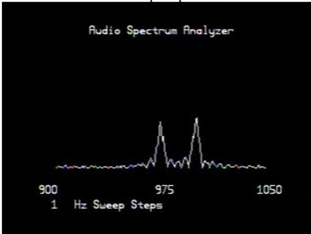
In this sample, the data was sampled for 100 Periods with an input frequency of 975Hz and 1000Hz. The sweep step was set at 1Hz intervals between 900Hz and 1050Hz
