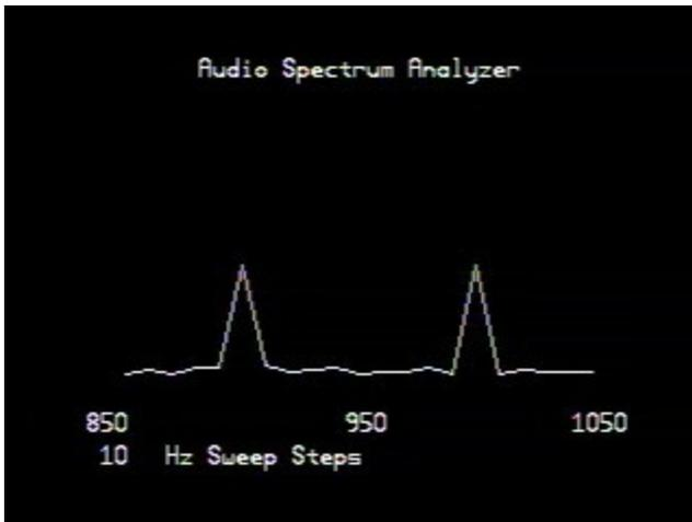
In this sample, the data was sampled for 100 Periods with an input frequency of 900Hz and 1000Hz. The sweep step was set at 10Hz intervals between 850Hz and 1050Hz. In other words a vertical ZOOM
