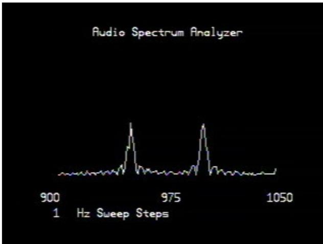
In this sample, the data was sampled for 100 Periods with an input frequency of 950Hz and 1000Hz. The sweep step was set at 1Hz intervals between 900Hz and 1050Hz
