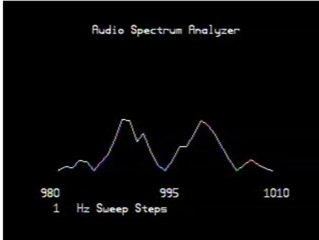
In this sample, the data was sampled for 100 Periods with an input frequency of 990Hz and 1000Hz. The sweep step was set at 1Hz intervals between 980Hz and 1010Hz
