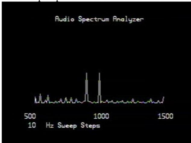
In this sample, the data was sampled for 100 Periods with an input frequency of 900Hz and 1000Hz. The sweep step was set at 10Hz intervals between 500Hz and 1500Hz
