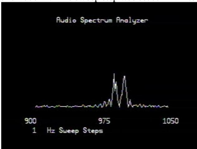
In this sample, the data was sampled for 100 Periods with an input frequency of 990Hz and 1000Hz. The sweep step was set at 1Hz intervals between 900Hz and 1050Hz
