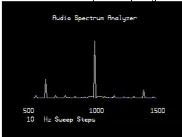
In this sample, the data was sampled for 100 Periods with an input frequency of 1000Hz. The sweep step was set at 10Hz intervals between 500Hz and 1500Hz
