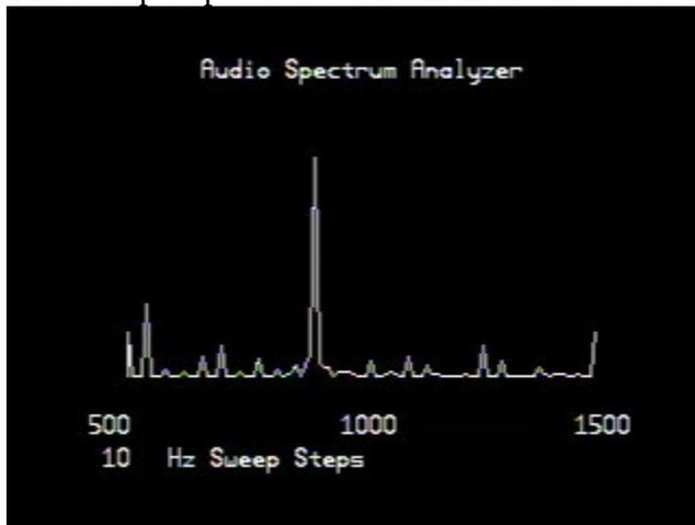
In this sample, the data was sampled for 100 Periods with an input frequency of 900Hz. The sweep step was set at 10Hz intervals between 500Hz and 1500Hz
